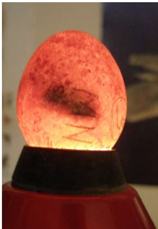
Photo 3. Ovoscope used to detect infertile eggs and the developmental stage of failed eggs. Infertile eggs have no embryo and do not show any dark spot, while eggs with dead embryos show a dark spot with a size depending on the age of the embryo (Aurora M. Castilla).
