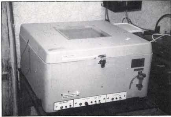
A. B. Incubator. With optional Auto overheat cut out.
