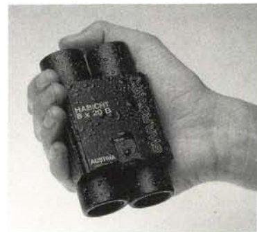
Water- and dustproof due to its interior focussing system. Neither focussing nor dioptic adjustment can cause the outer lenses of the binocular to be moved, i.e. the entire optical system is thus hermetically sealed against water and dust.
