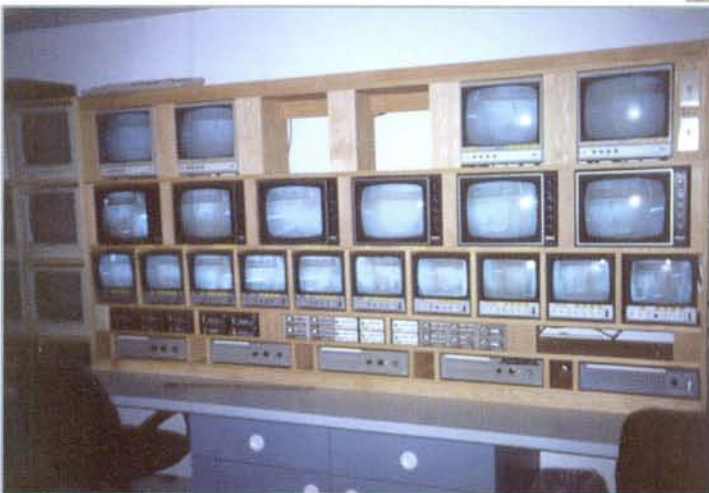
Bank of Video monitors which are connected to each breeding chamber. Photo: Bruce Haak
