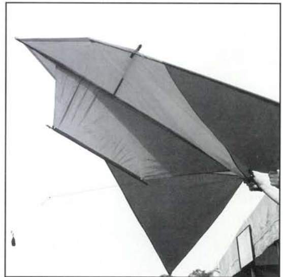
A typical Nylon Delta Kite. These are very light and strong, using modern carbon fibre and fibre-glass.
