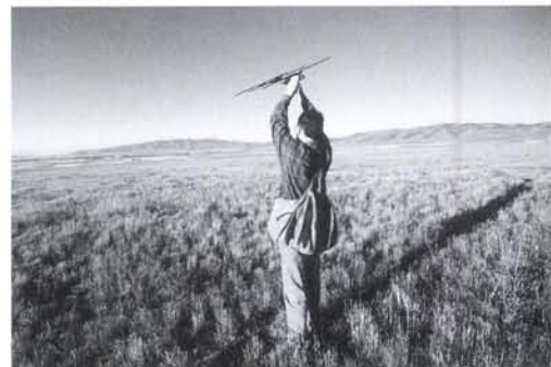
Figure 3 - When tracking a weak signal hold your antenna as high as you can reach.
