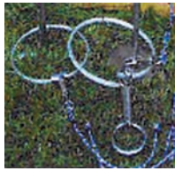
Spring swivel tether. Launched 1997. 1st effective shock absorber designed for tethering Raptors.
