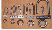
Clockwise from left: Cheap swivels, Individual elements, The finished product, Welding tool
