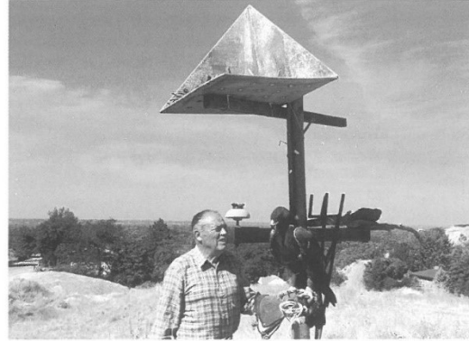
Morlan Nelson with some of the mock-up powerpoles and proto-type nest platforms.
