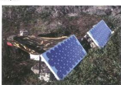
Photo 3. The solar panel array, battery bank (in black action packer), and recording system (gray pelican case covered by camouflage tarp) located at the top of a nesting cliff.
