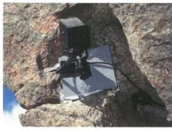
Photo 2. View of the small camera glued to the rock wall at an eyrie.
