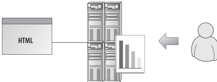
Figure 2.2 Schematic logfile methodology: The web server logs its activity to a text file that is usually local. The analytics customer views reports from the local server.
