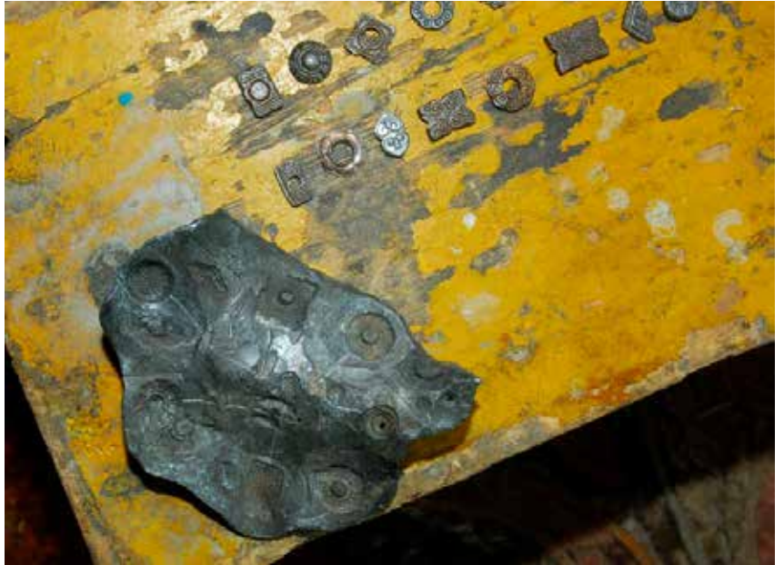
Figure 3. Traditional rivet designs and the pattern iron pedestal
