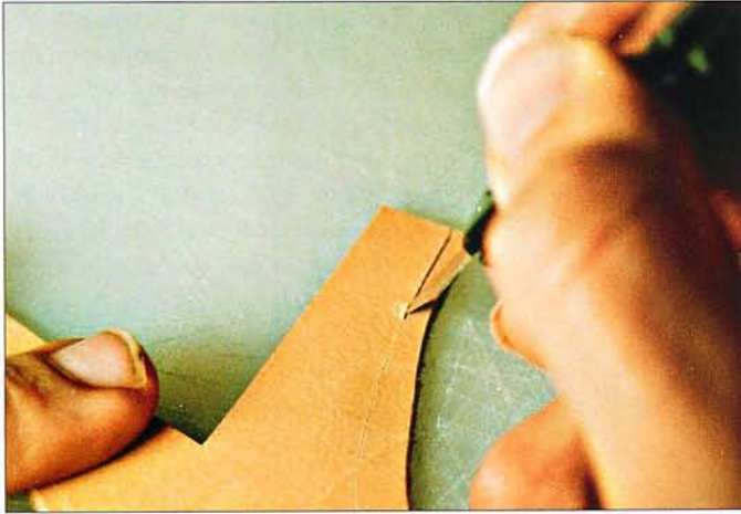
Figure 1: Cutting the seams at an angle.
