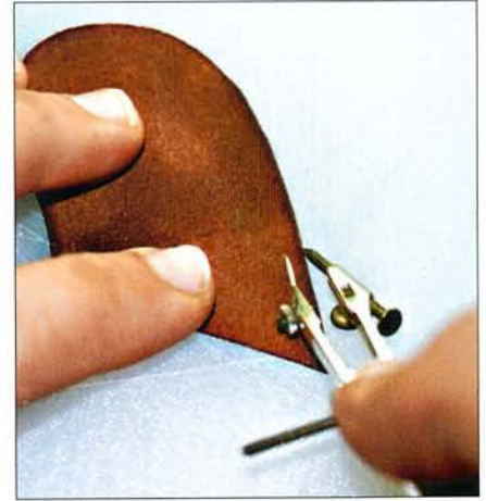
Figure 2: Marking the stitch tracks with a set of compasses.
