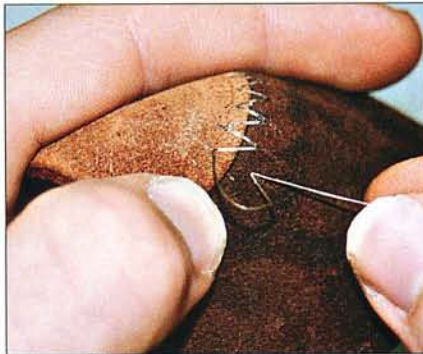
Figure 8: Holding the hood while sewing.
